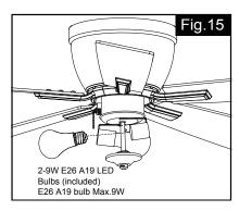
Install LED bulbs (included). See relamping label at socket area or packaging for maximum wattage allowed.
