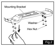
Unscrew the washers and hex nuts from mounting bracket.
