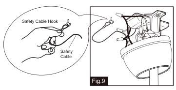
Hang the safety cable into the safety cable hook.
