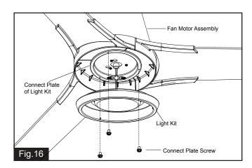
Remove three connect plate screws from connect plate of light kit first (for later use). Then connect the white (neutral) wire from the light kit to white (neutral) wire from fan motor assembly with a wire connector; connect the black (hot) wire from light kit to blue (hot) wire from fan motor assembly with a wire connector. Carefully put the wires into the connect plate of light kit, then attach the light kit onto the connect plate of light kit with the connect plate screws.
