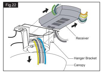
Unscrew the canopy. Remove the wire connectors from the fan to ceiling wire connection. The receiver should be removed from the hanger bracket. (See Fig.22)
