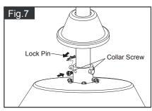
Insert the two collar screws into the collar until tight. Slide lock pin into hanger pin until it is locked into position.
