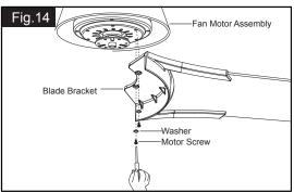
Remove the motor screws and washers from the fan motor assembly. Secure blade brackets to the motor with washers and motor screws.
