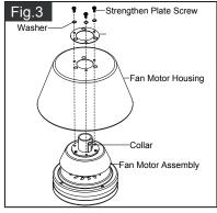
Align and engage the fan motor housing and strengthen plate to the fan motor assembly. Then secure the strengthen plate to the fan motor housing with washes and strengthen plate screws.
