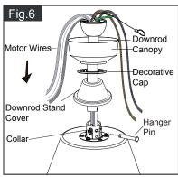
Insert the downrod into the collar. Slide hanger pin through holes of collar and downrod.
