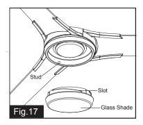
Attach the glass shade to the light kit by aligning studs and slots, and turn clockwise until it is locked in place.
