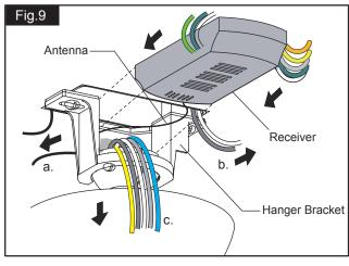
Move ground wires (a), outlet box wires (b), and motor wires (c) way from the center of the hanger bracket as shown. Thread the antenna through the hanger bracket first, then thread the receiver through the hanger bracket until it is placed in the center. Finally, cut motor wires (c) to length needed for connections.
